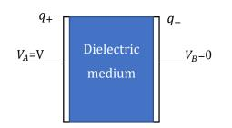
Let the space between the two plates of the capacitor is filled with a dielectric medium of dielectric constant K.
