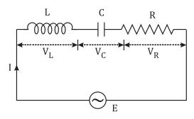
Let E and I be the instantaneous values of e.m.f. and current in the LCRcircuit; and  $V_L$ ,  $V_C$  and  $V_R$  be the instantaneous values of the voltages across inductor L, capacitor C and resistor R respectively. Then,  $V_L = IX_L$ ;  $V_C = IX_C$  and  $V_R = IR$
