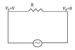
$dH = I^2 R dt = (I_0 \sin \omega t)^2 R dt = I_0^2 R \sin^2 \omega t dt$ The amount of heat produced in the resistance in time T/2 (half time period) can be obtained by integrating the above equation between the limits t = 0 to t = T/2 i.e.
